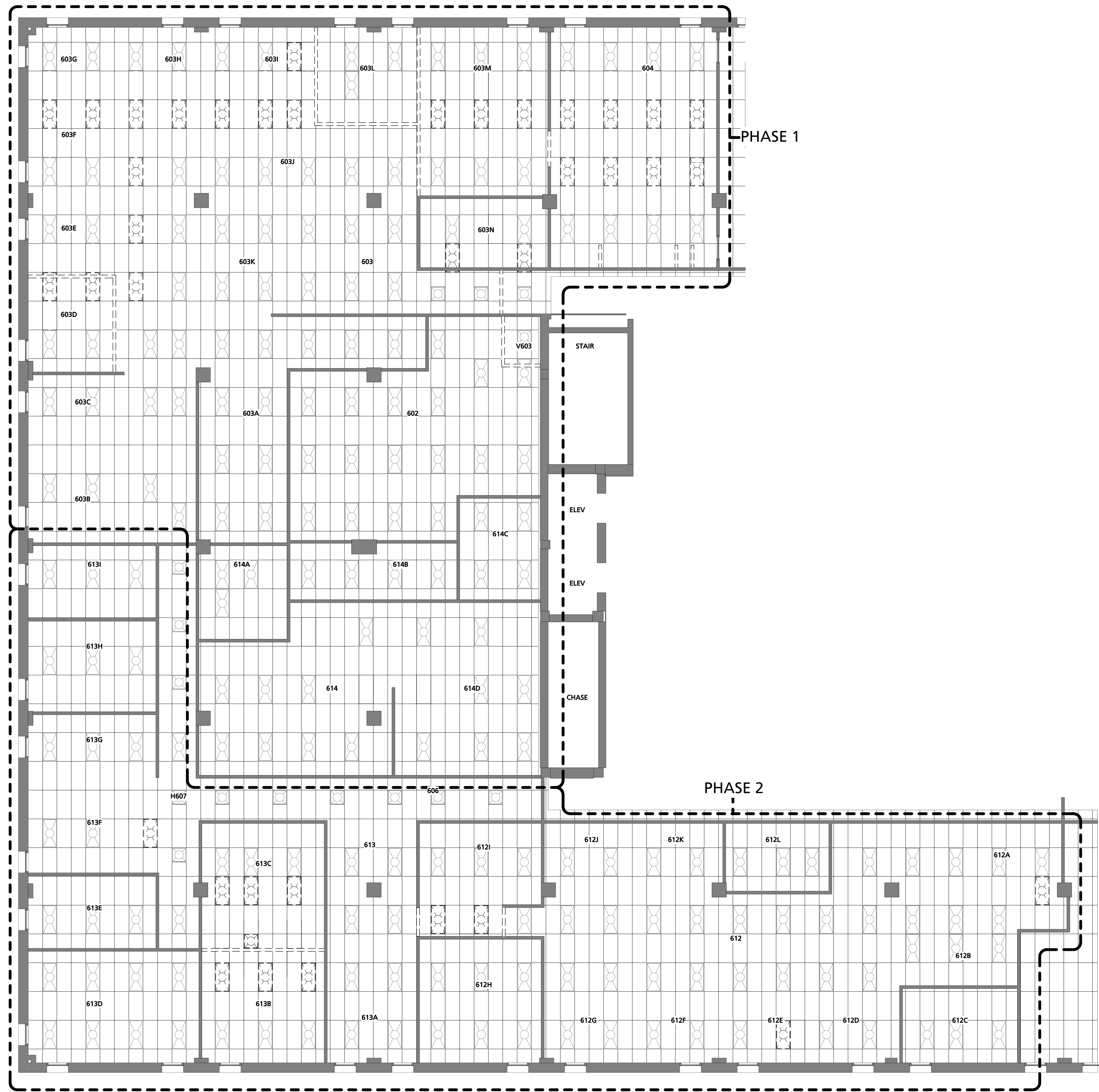
1 SIXTH FLOOR-DEMOLITION PLAN 1/8" = 1'-0"
